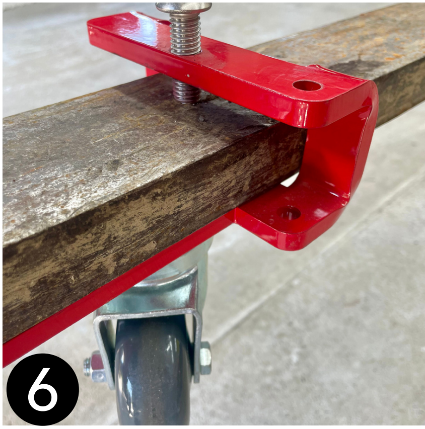
Install fork dolly onto forks
