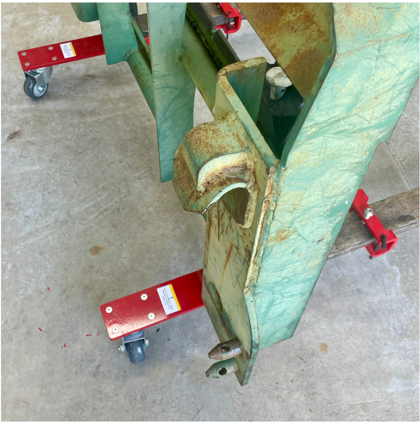
Fork dolly must go past the fork frame mount as pictured above
