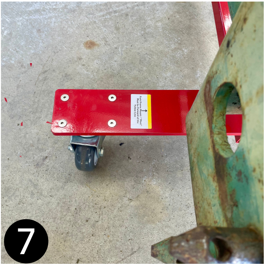
Fork dolly must go past the fork frame mount as pictured above
